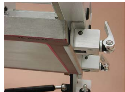
Fast slide-in clamping of frame Slide-in clamping with fixed width.
