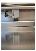
Pneumatic clamping of print frame with thickness up to 40 mm.
