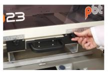
Adjustable clamping of the frames from 12" to 23" width
