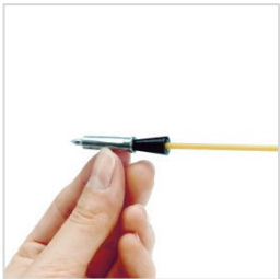
Cleaning of dispensing nozzles with special adapter
