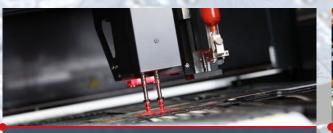
Configurable heads with 1-4 placement-axis. 2,5D and 3D dispensing and jetting, High resolution digital vision system with auto component teach-in and irregular ball recognition.
