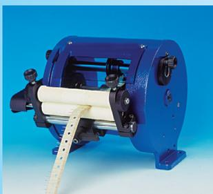
TNS - 21.0011 ESPULSORE NASTRO DI SCARTO
