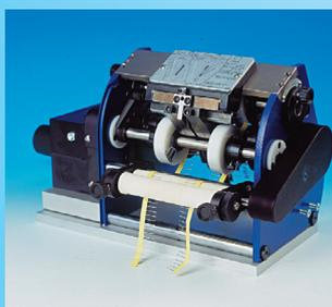
TNS - 21.0013 ESPULSORE NASTRO DI SCARTO
