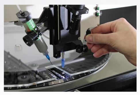
Being able to adjust the placement force and avoid operator fatigue, this unique feature allows precise placements even after long working periods.
