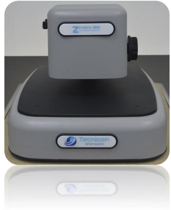
With any inspection type machine data analysis is paramount. The Z-Check 100 has as standard a comprehensive SPC package. With the vast array of PCB's that the Z-Check is able to handle, the user has the option of 10 production lines with unlimited products within those lines to choose from, creating a large library of data.
