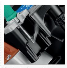
JBC Fume Extractor has an integrated vacuum system that detects when the tool is returned to the stand and automatically absorbs excess of fumes.
