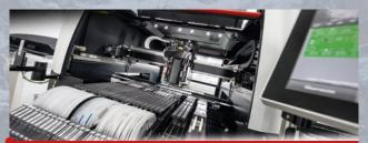
Configurable heads with 1-4 placement-axis. 2,5D and 3D dispensing and jetting, High resolution digital Cognex vision system with auto component teach-in and irregular ball recognition.
