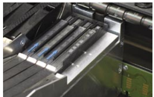
By changing the adapter (black) the stick feeders can quickly be fitted to different component dimensions.
