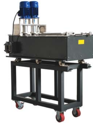
Solder pot independent designed, convenient for the cleaning and the change between normal and lead-free alloy
